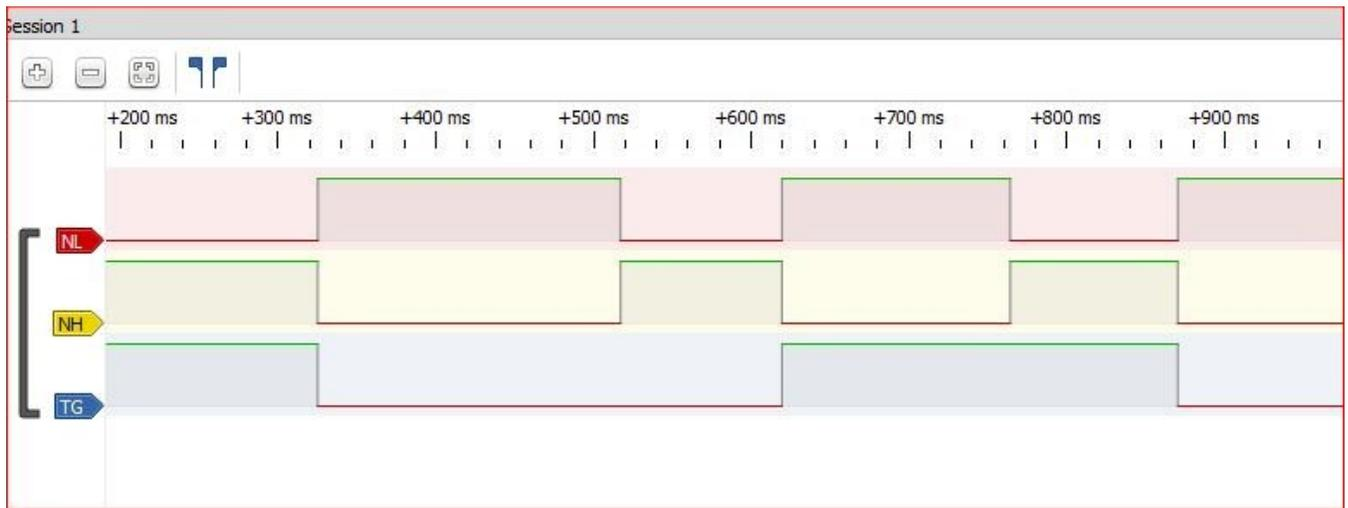
**Logic Analyzer Capture of the NL (Normally Low), NH (Normally High), and TG (Toggle) outputs of LSVR Switch**
