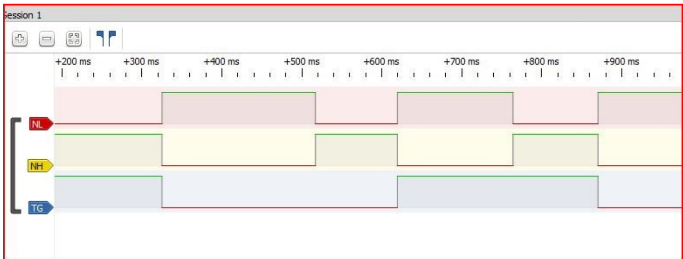
Logic Analyzer Capture of the NL, NH, and TG outputs of LSVR Switch
