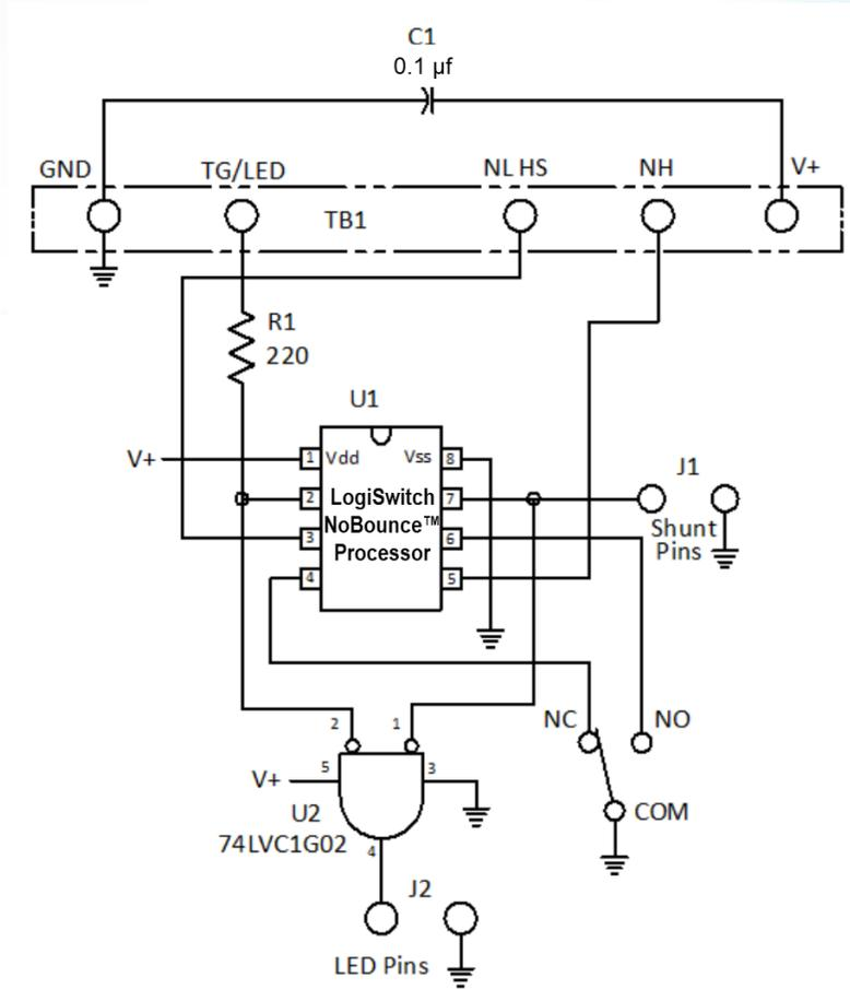
LS-22 mm NoBounce Pushbutton Switch Schematic
