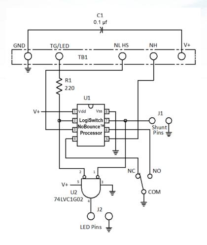
LS-22 mm NoBounce Pushbutton Switch Schematic
