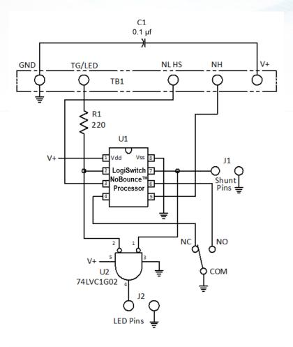
LS-19 mm NoBounce Pushbutton Switch Schematic
